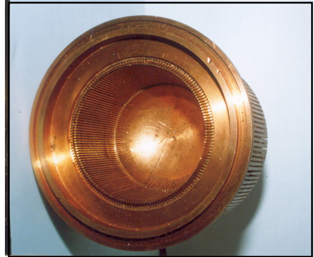
Figure 3: Pictorial view of flawless Cryogenic condenser ready for assembling
